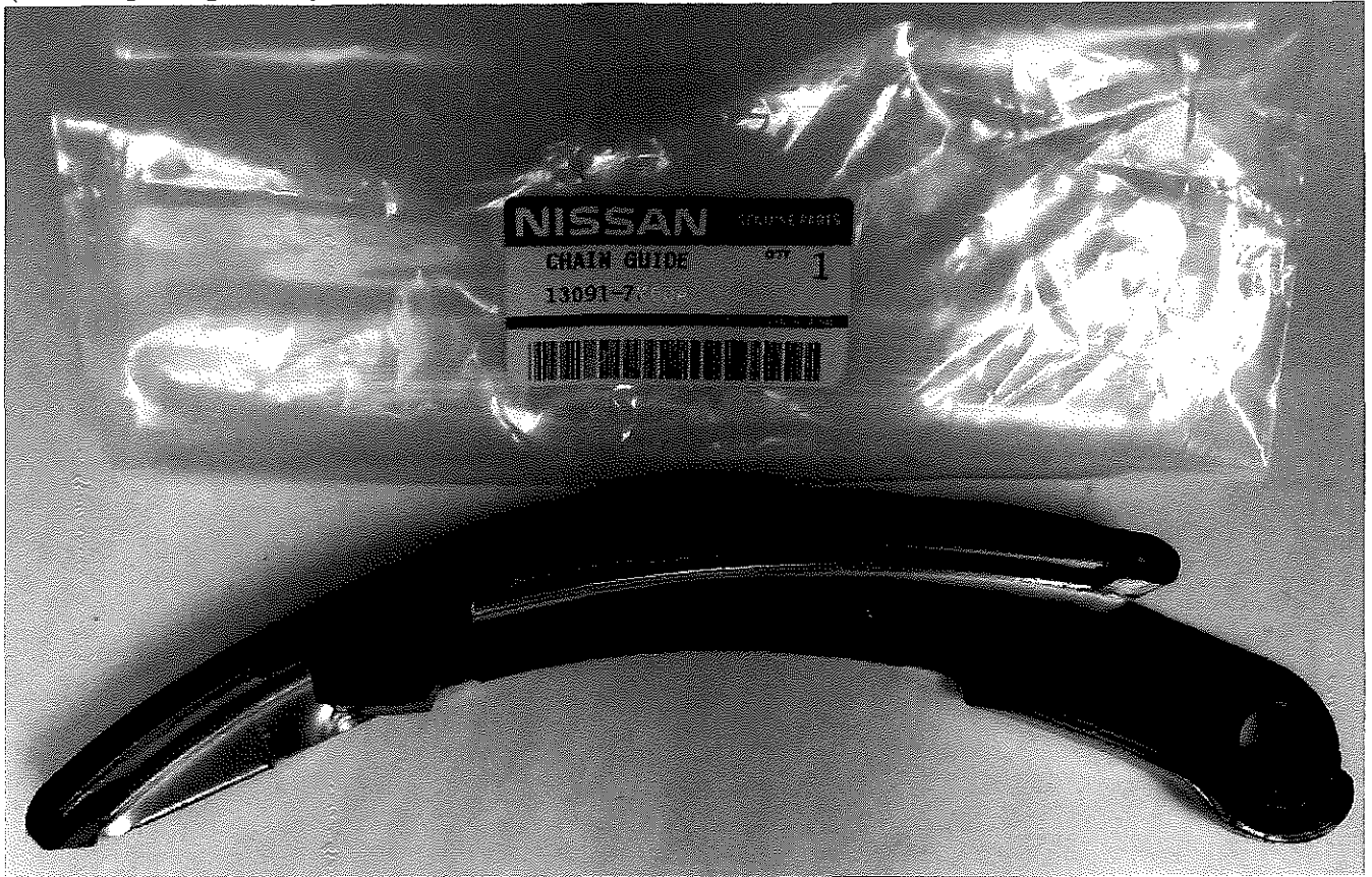
Figure 7: (Redesigned primary timing chain guide, Nissan Part Number 13091-ZK00A)
