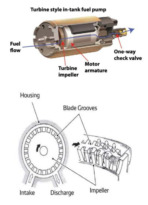
32.3 The fuel pump assembly and all its components are always exposed to gasoline within the fuel tank. Fuel pumps are designed to survive the harsh environment for at least 320,000 kms (200,000 miles). DENSO claims that its fuel pumps "offer more than triple the lifetime...", the whole as appears more fully from a copy of the Autoblog article entitled "How Long Does a Fuel Pump Usually Last?" dated
