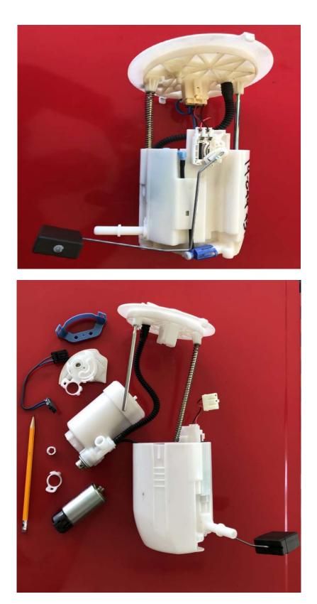
32.5 The fuel pump module's housing protects the fragile internal components that fit together very specifically (<u>like puzzle pieces</u>) within the module and is held together with plastic tabs and clips:
