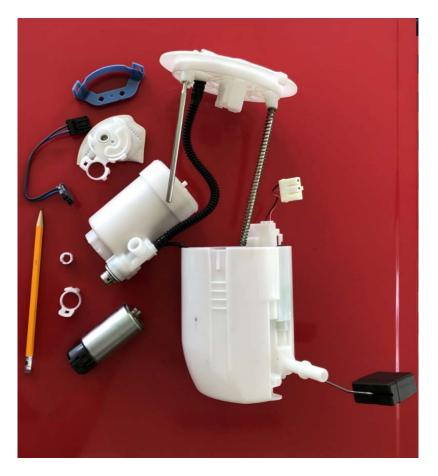
45. The fuel pump module's housing protects the fragile internal components that fit together very specifically (like puzzle pieces) within the module and is held together with plastic tabs and clips:
