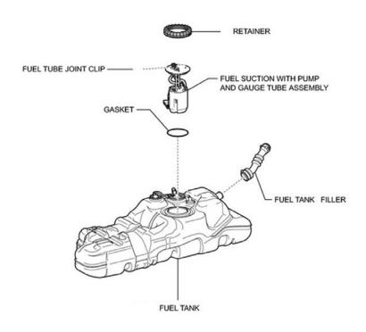
44. The fuel pump (i.e., the electric motor and impeller) is an internal component of the fuel pump module. The fuel pump module hosts the fuel pump, associated plumbing and the fuel gauge sending unit. The fuel pump module drops into the fuel tank through an access hole on the topside of the tank. A retainer ring ensures that the flange<sup>3</sup> and O-ring create a tight seal against the tank surface, preventing fuel escape:
