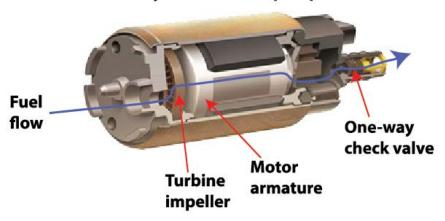
42. DENSO explains the role of the electric fuel pump as "deliver[ing] fuel from the tank to the engine, under high pressure, depending on the vehicle application's specific requirements. The fuel is transported to fuel injectors, which spray the fuel into the engine cylinders" (Exhibit P-15);
