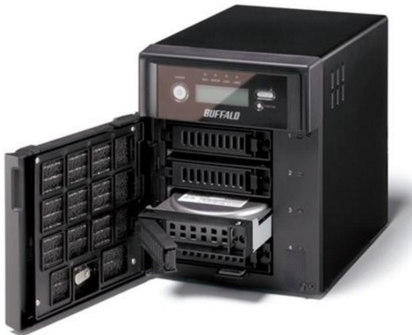
14 *Figure 1: Network-Attached Storage device.*
